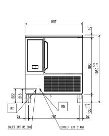
Drain Electrical inlet (power) ΕI Refrigerant Outlet
